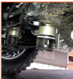
Shows 2 main spacers installed from rear view
